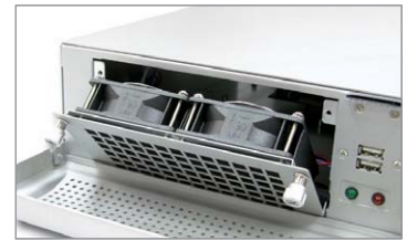
Front Replaceable Air Filters/Fans
