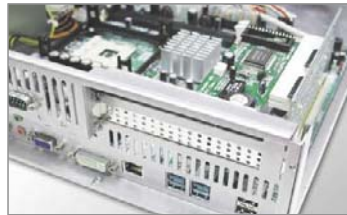
PCI Expansion Two PCI expansion slots for adding more functions to the system
