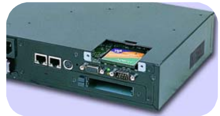
External assessable Compact Flash socket
