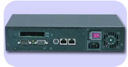
Flexible I/O panel for different boards
