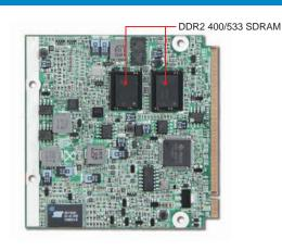
Portwell PQ7-M102XL is designed with Intel's ultra low power US15WPT chipset which features less then 5W overall power consumption and -40~85 degree wide temperature support. It is suitable for intelligent grid technology applications to control and monitor smart meter and to integrate the electricity from wind and solar power for more efficient usage of energy to the country.
