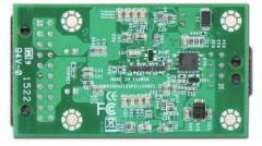
GADIWA-B1120 is a DC to DC 12V input board type converter. It normally support continuous 120 Watts and peak 160 Watts.
