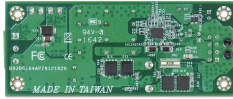
GADIWA-R9142 is a DC to DC 9V~32V input to 24V output board type Regulator. It normally support continuous 140 Watts and peak 160 Watts. GADIWA-R9142 can save more space, less than 1U width, and cost. It's not only capability for fan-less system but also suitability for different applications. Besides, the converter is made and tested by automatic production line; therefore, it can provide high quality and better performance.
