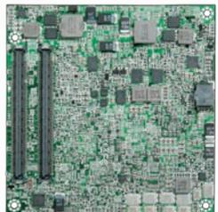
The Portwell PCOM-B219VG is designed with the Intel® QM77 express chipset which offers high computing power with the 3<sup>rd</sup> generation Intel® Core™ family. This provides turbo-boost, vPro, Hyper Threading, 3D Tri-gate Transistors, USB 3.0 and all the other materials necessary of withstanding wide temperature ranges necessary for harsh environment.
