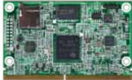
PSMC-M310T is design as CPU module series with SMARC form factor. It is based on embedded TI™ AM3354 Single-core processor, an ARM® Cortex®-A8 processor. Best cost-effective entry model to replace original markets of ARM9 and ARM11.
