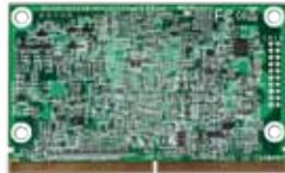
The SMARC (“Smart Mobility ARChitecture”), small form factor of lower power, cost concern, and high performance, is used as building blocks for portable and stationary embedded systems. The SMARC pin-out is optimized for the features common to ARM CPUs and not common to the x86 PC world. The modular approach allows scalability, fast time to market and upgradability while still maintaining cost performance, low power and small physical size.
