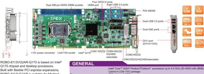
Q170 chipset and desktop processors. Built with flexible PCI express expansions, ROBO-8113VG2AR is suitable for Medical, Industrial automation, and Digital Signage application.
