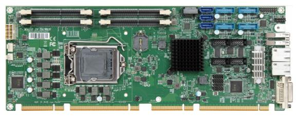
ROBO-8114VG2AR-Q370 is based on Intel® Q370 chipset and desktop processors. Built with flexible PCI express expansions, ROBO-8114VG2AR-Q370 is suitable for Medical, Industrial automation, and Digital Signage application.
