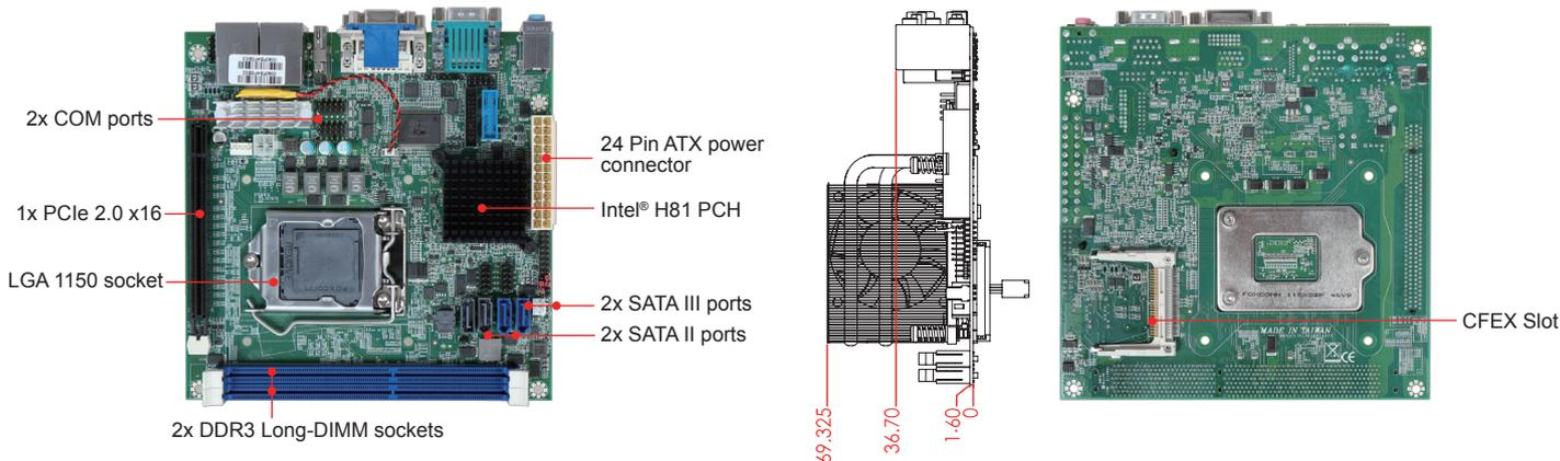
WADE-8016 is based on Intel® H81 chipset and desktop processor sku like Core™ i7 and i5. WADE-8016 of the Intel® platform will provide high performance and flexibility for functional expansion, such as Gaming, Kiosk, DS, Medical, Defense, Industrial automation and control applications.
