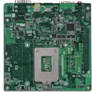
WADE-8210-H110 is based on Intel® H110 chipset and Desktop processors including Intel® 7<sup>th</sup> and 6<sup>th</sup> Gen Core™ i3/i5/i7 SKU. This board supports DDR4, PCIe 3.0, and SATA III. Those features help you to build high performance and stable system.
