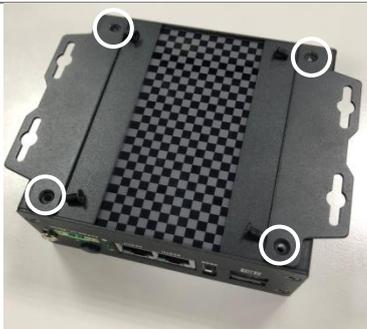
**Step 2.** Choose the correct type of mounting surface and securely attach the LYNX-6000 series on it (desk/wall). Ensure that the attaching hardware is in the small section of the keyholes.
