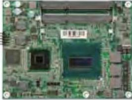
Intel® 4<sup>th</sup> Generation Core™ i7 Processor based on Type VI COM Express module with DDR3L SDRAM, VGA, LVDS, Gigabit Ethernet, SATA 3.0 and USB
